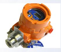
Flamgard Plus is a Flameproof (Ex d), ATEX, IECEx and UL certified flammable gas detector, which uses poison-resistant pellistors to detect explosive levels of hydrocarbons, hydrogen and other flammable gases and vapours, including aviation fuel and leaded petrol vapours.
