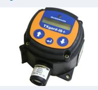
TXgard-IS+ is an Intrinsically Safe (I.S.), 2-wire, toxic and oxygen gas detector with local LCD display. A wide choice of sensors is available for use in a variety of applications. TXgard-IS+ is ATEX and IECEx certified for use in Zone 0,1 or 2 hazardous areas, and also UL and cUL certified for use in Division 1 or 2 hazardous areas.
